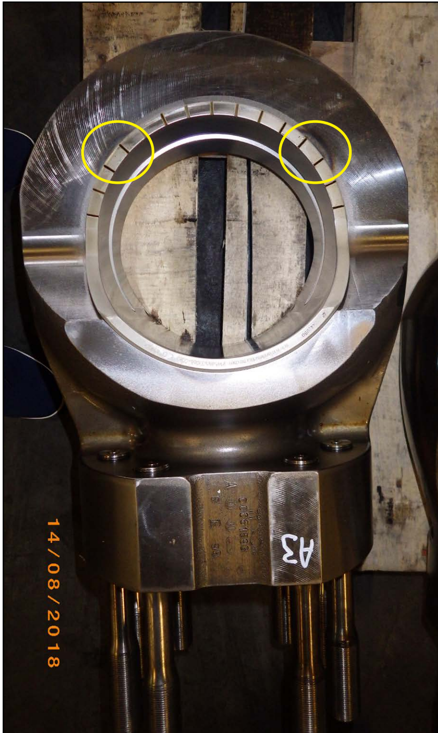
Figure 27: Botnia Seaways small end heat damage (circled)
