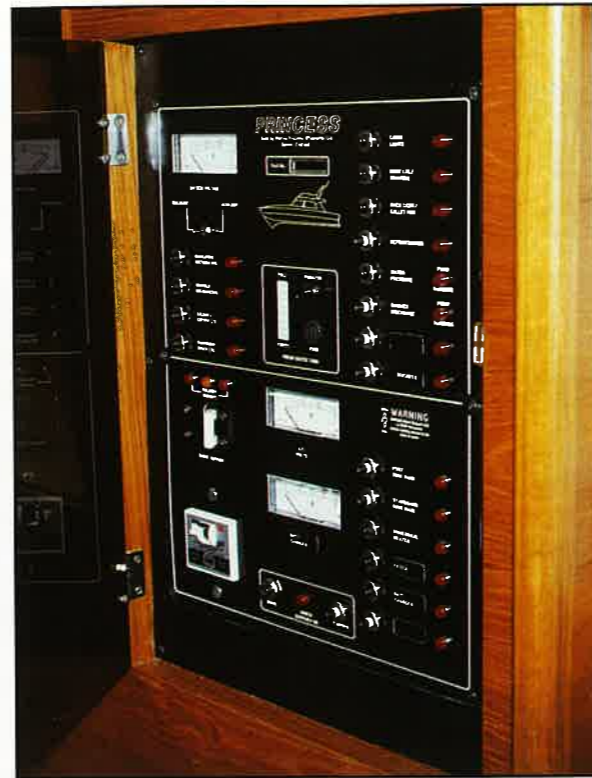
Left: access to the Volvo diesels under the saloon floor is simple. Above: an electrical distribution board is neatly set into the helm seat.
