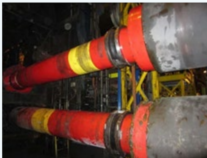
Photographs 6a and b- Strain Gage Telemetry System Installation on shear spacer (left) and permanent installation on counter-rotating shafts (right).
