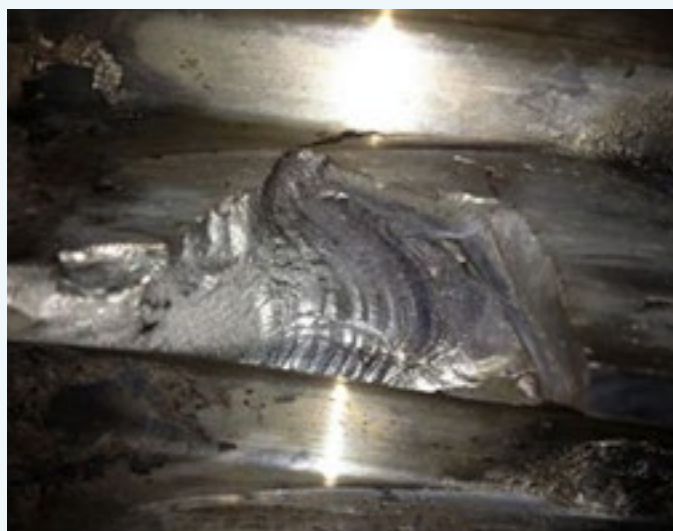
Photographs 5a and b: Fatigue failure surfaces of shear pin subjected to cyclic stress below the prescribed overload limit but above the material endurance (left) and fatigue fracture of a crowned gear tooth from repeated impacting (right).
