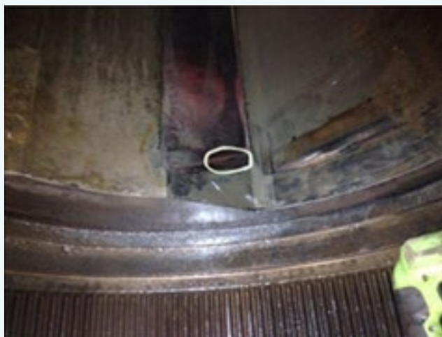
Photographs 7a and b: Inspection of drivetrain component subject to repeated high torques in Figure 11. Cracks located in the area shown (left) were detected using magnetic particle inspection (right).
