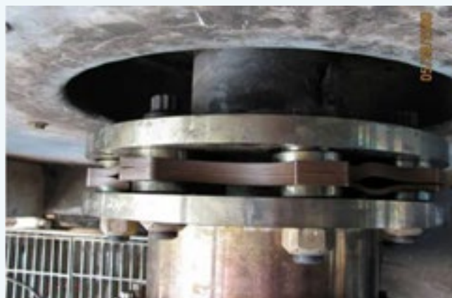
Photographs 4a and b: Inspection of coupling element (disc pack style) showing minor distortion due to slight overload (left) and severe buckling of discs (right). Note that deformation/buckling occurs in the centre of the link between alternating bolted connections.
