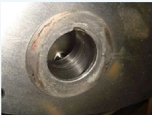
Photographs 2a and b: Showing fretting wear around bolt hole from dynamic contact with mating washer (left) and crack initiated in fretting zone (right).
