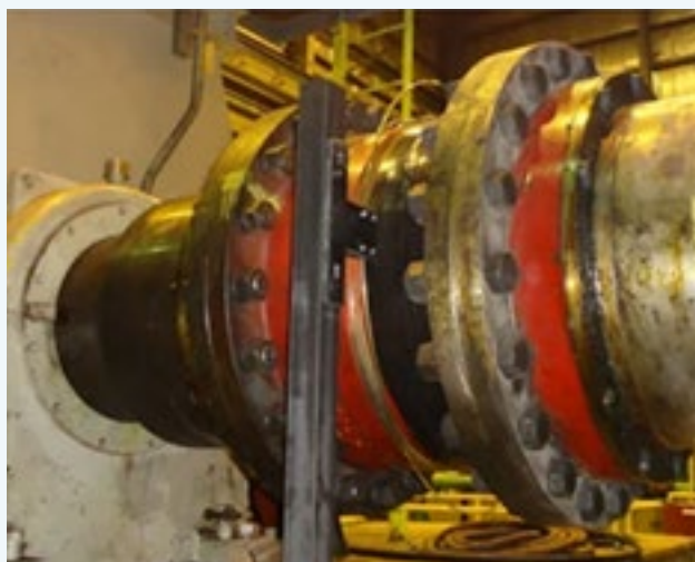
Photographs 6a and b- Strain Gage Telemetry System Installation on shear spacer (left) and permanent installation on counter-rotating shafts (right).
