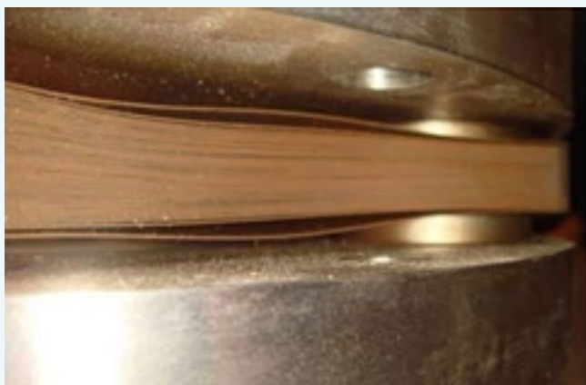
Photographs 4a and b: Inspection of coupling element (disc pack style) showing minor distortion due to slight overload (left) and severe buckling of discs (right). Note that deformation/buckling occurs in the centre of the link between alternating bolted connections.
