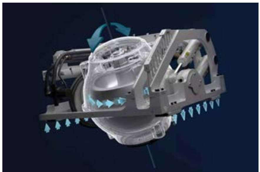
The gyro stabiliser works by spinning the flywheel ~which endeavours to remain horizontal.
