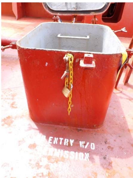
Figure 3: Aft booby hatch for Cargo Hold No. 1.
