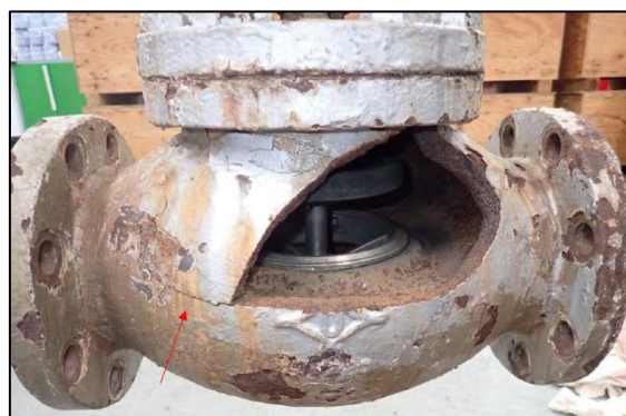
Figure 7: Continuing crack with further existing cracks bifurcating from it
