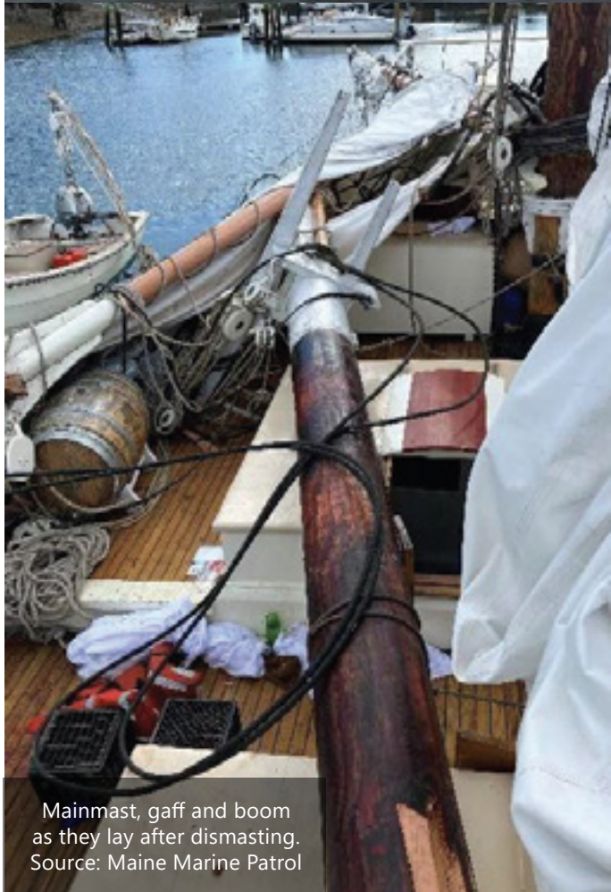
Main gaff resting atop the main boom. Source: USCG
