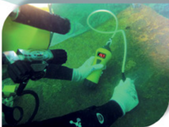
The Underwater Thickness Gauge MultigaUGE 3000
