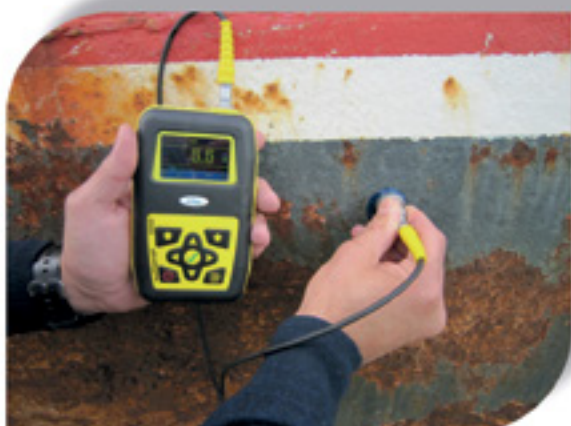
The Surveyors Thickness Gauge MultigaUGE 5650
