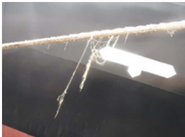
Figure 11.1 Mooring line degradation
