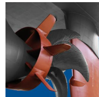
Becker Mewis duct twisted (~3-8 % power saving)
