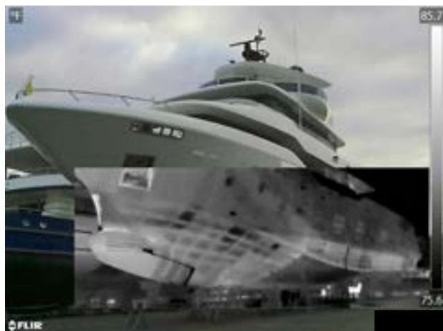
Hull bottom inspection using a Teledyne FLIR f=5\text{mm} ( 80^\circ ) Field of View (FOV) wide-angle lens.
