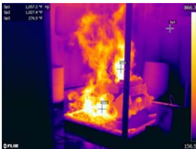
Marine inspection of a controlled engine room fire. The thermogram was displayed using the Ironbow color palette, providing distinct, informative, and accurate thermal interpretation.
