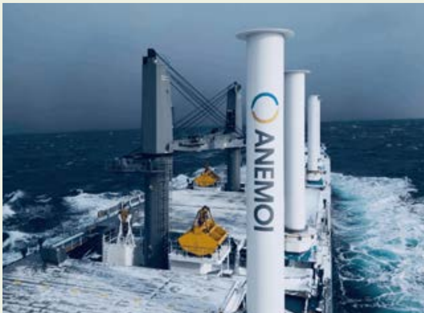
Four Anemoi Rotor Sails demonstrating the wind-assisted propulsion system in operation
