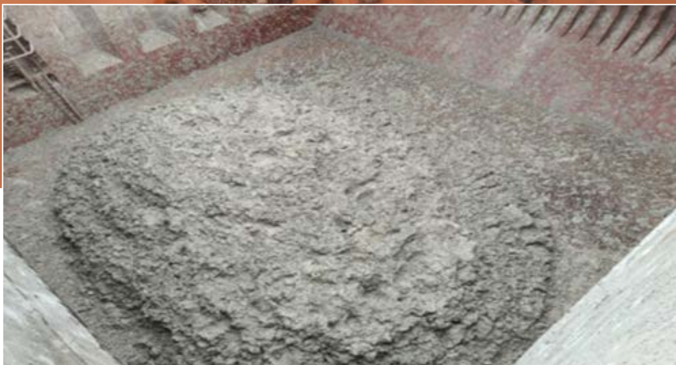
Clay cargo showing signs of splattering and flattening in cargo hold (Photo credit: SPICA)
