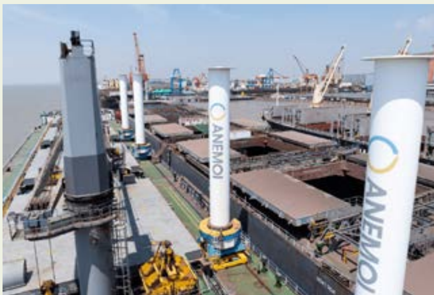
Wide view of M/V Afros in dry dock showing the Anemoi Rotor Sails and cargo handling areas
