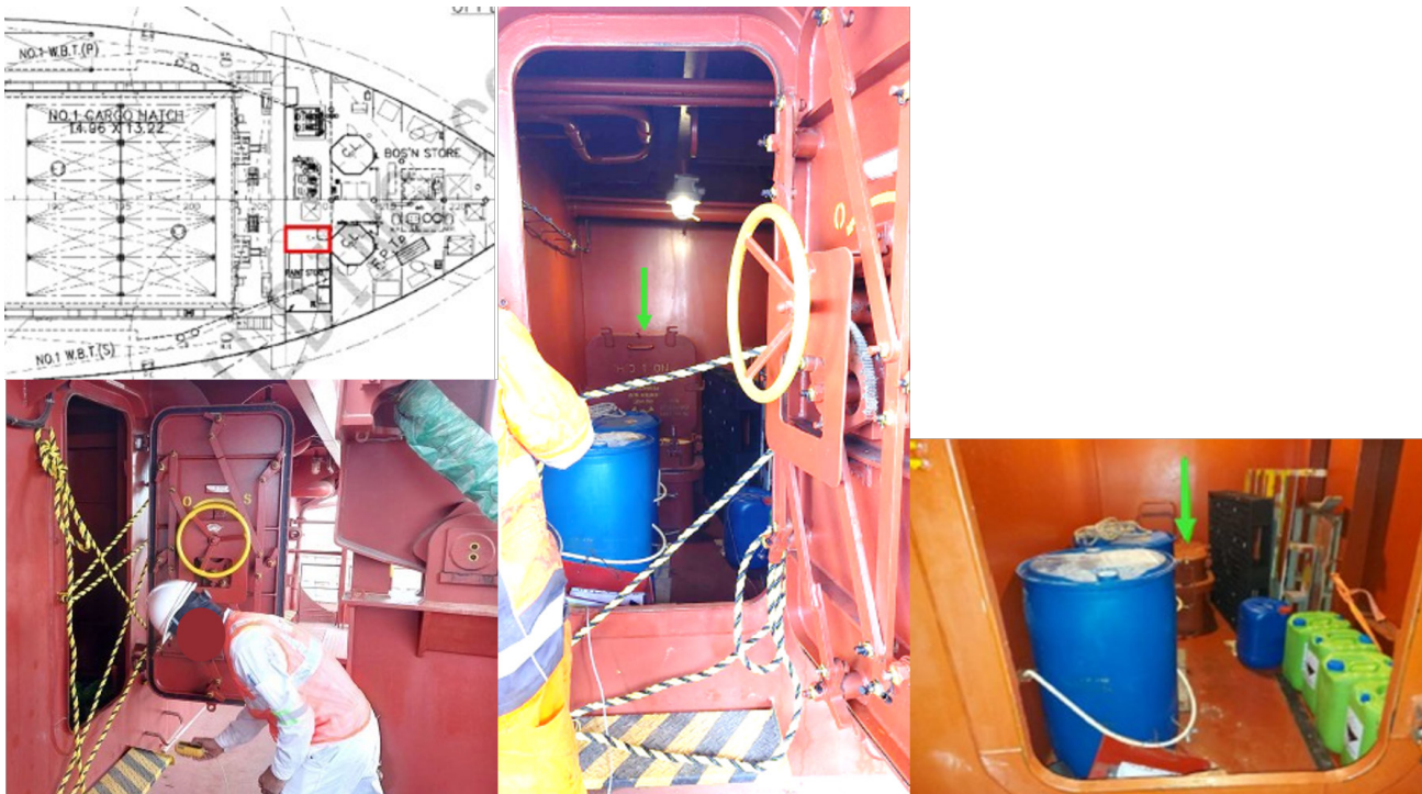
Figure 2: The CH No. 1 Access Space is indicated in red on the General Arrangement. The bottom left picture shows the location of the weather tight access door with the handwheel identified by the yellow circle. The green arrows in the middle and right pictures point to the booby hatch at the back of the space.
