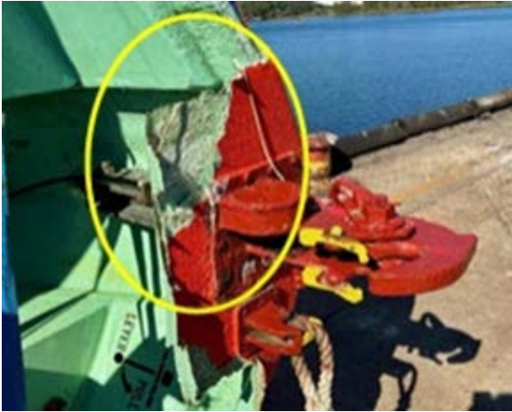
Damaged hook: Photo credit: U.S Coast Guard
